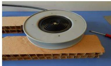
8) Insert the hub and hook the central spring lug onto the slot in the hub.
