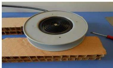
9) Screw the center screw inside the hub.
