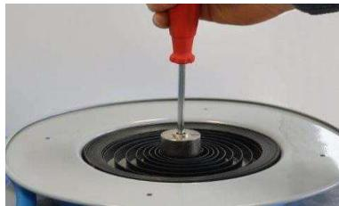
10) Fit the spring cover and tighten the four M4 screws.
