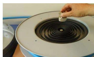
9) Tighten the center screw inside the hub, if present.
