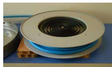
8) Fit the hub and hook the center spring lug to the hub slot.
