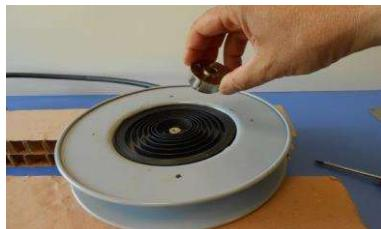
10) Insert the spring protection cover and tighten the four M4 screws.
